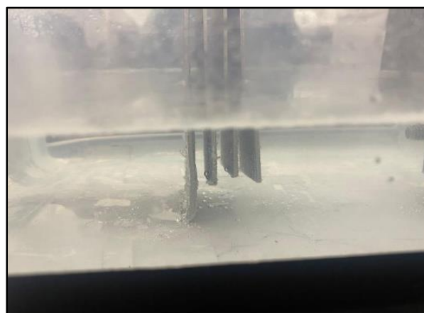
Fig. 5.2: Bubbles of Hydrogen generated within seconds of the supply voltage
