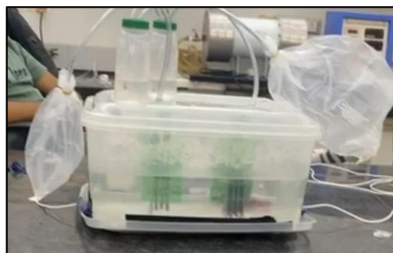
Fig. 5.1: Set-up of Hydrogen generation electrolytic cell
