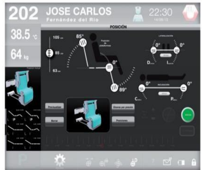
Fig. 4: Touch screen design control interface at the bedside [5]
