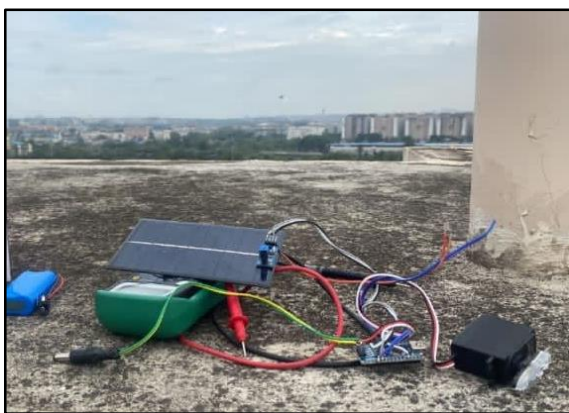
Fig: 3.2: Image representing the Solar Panel Set-up for Solar Tracker Methodology
